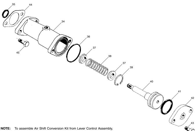
omit Shifter Ball, Spring, Cylinder End Oil Seal, Jam Nut and Eye Bolt.
