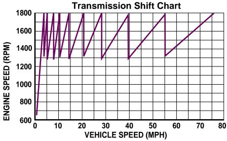
T-310 w/1800 RPM ENGINE, REAR RATIO 3.86 AND 11R22.5 TIRES (BASED ON 504 TIRE REVS PER MILE)
