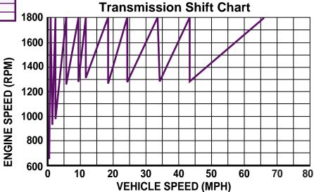
T-310MLR w/1800 RPM ENGINE, REAR RATIO 4.64 AND 11R22.5 TIRES (BASED ON 498 TIRE REVS PER MILE)
