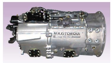
highway cruising. PTOs can be driven from both fixed and speed dependent mounts on all models. (For applications which require backing control and a slow 28.98:1 reverse ratio, refer to the data sheet on the T-318LR21.)
