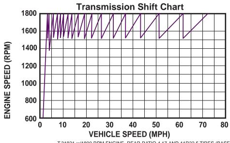
T-31821 w/1800 RPM ENGINE, REAR RATIO 4.17 AND 11R22.5 TIRES (BASED ON 504 TIRE REVS PER MILE)
