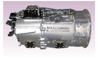
way cruising. For applications which require backing control, the LR model features a slow 28.98:1 reverse ratio. PTOs can be driven from both fixed and speed dependent mounts on all models.
